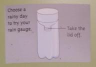
1. Cut the top third off a large plastic bottle. Upturn the top part and put it inside the bottom part. Stand it outside.
